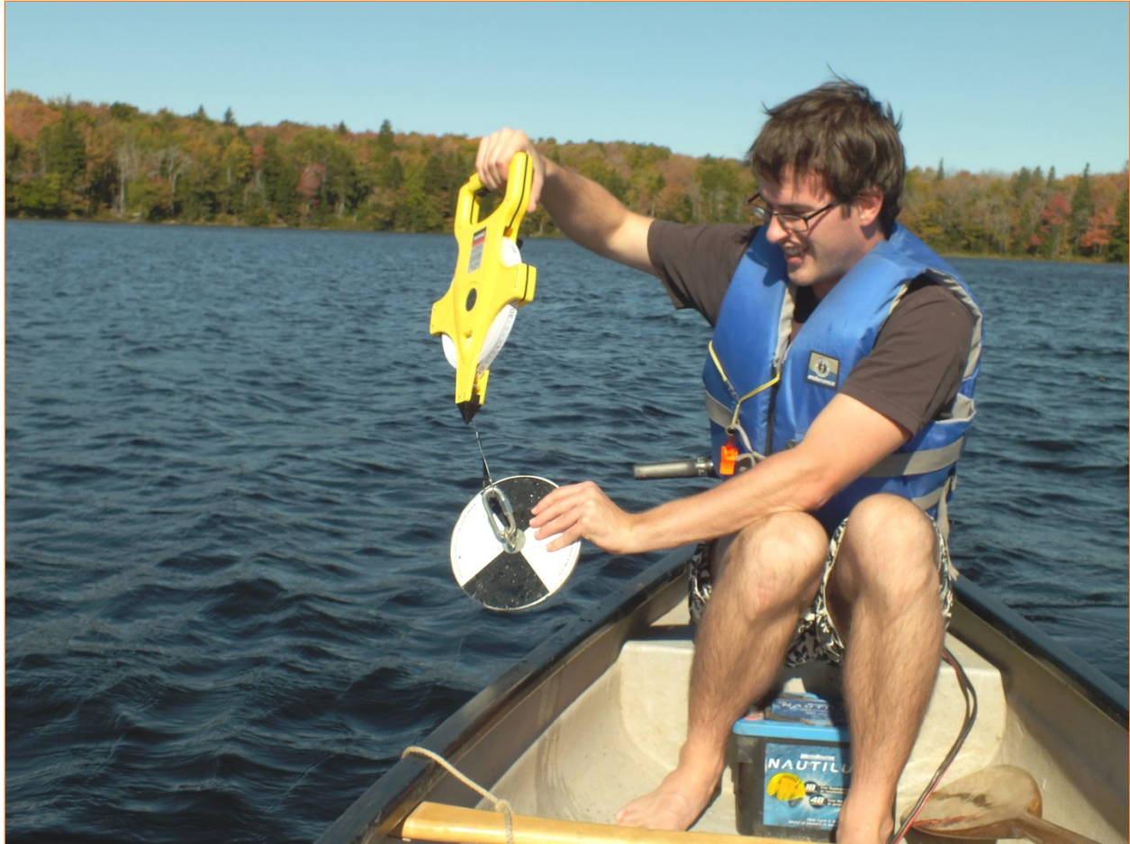
FIGURE 2-1 A SECCHI DISK USED TO TAKE A SECCHI DEPTH READING AT MONITORED LAKES
